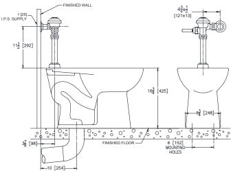
Rough-in/Overview dimensions for Z5655 Series Z5665-BWL1 with top spud Z5666-BWL1 with top spud and bedpan lugs
